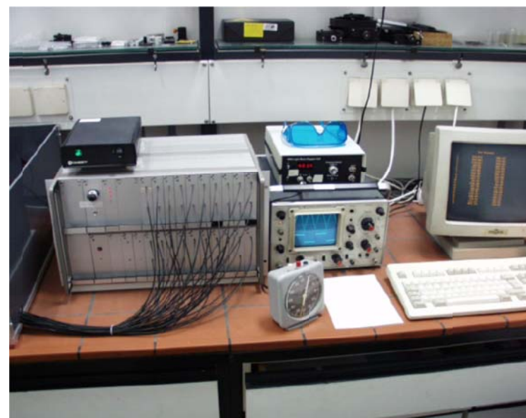
Fig. 2: Light guides are connected to photodiodes inside the grey box.
